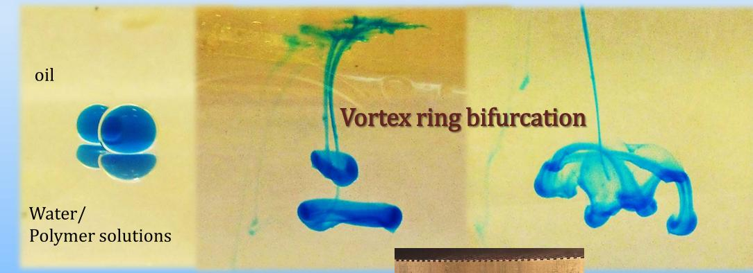
**PO120:** Hydrodynamic focusing of low viscous liquids and weakly elastic polymer solutions
